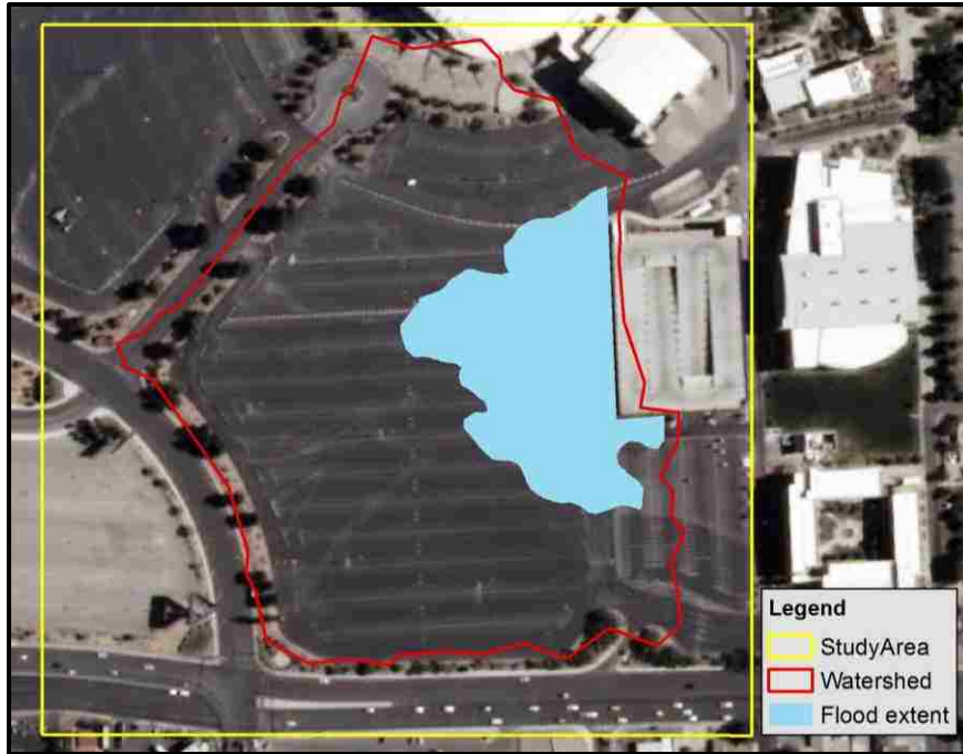
Figure 5.1-16: Inundation extent at 60 minutes after rainfall in Blacklot watershed
