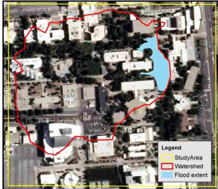
Figure 5.2-13: Inundation extent after 60 minutes of rainfall in East Mall watershed
