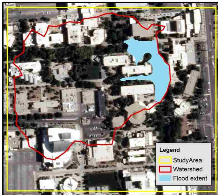
Figure 5.2-16: Inundation extent after 650 minute of rainfall in East Mall watershed
