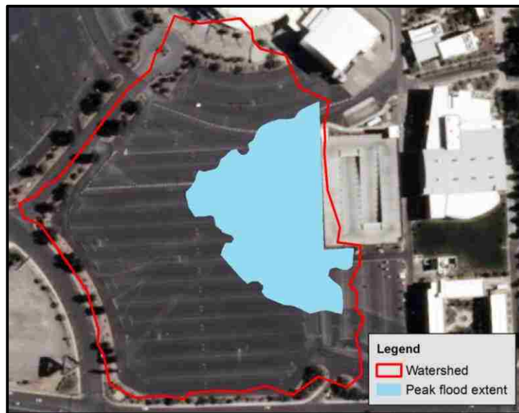
Figure 6.3-6: Peak inundation extent for gravel swale strip
