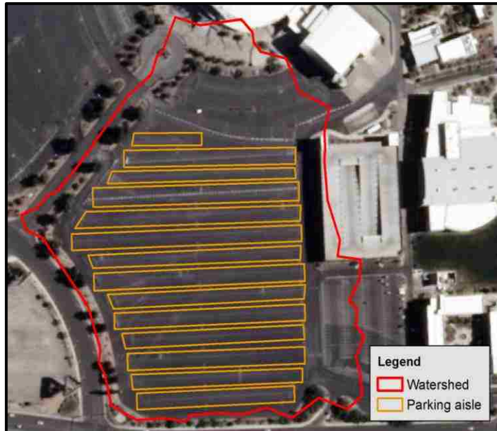
Figure 6.2-4: Schematic presentation of parking aisle filled with grass pavers
