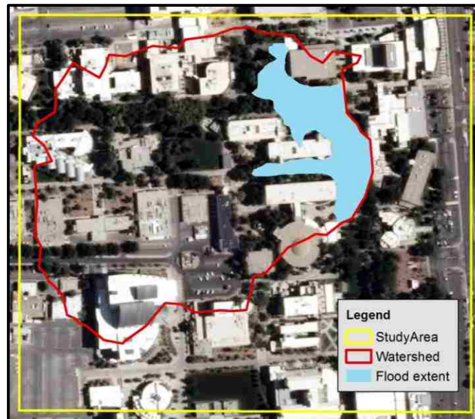
Figure 5.2-14: Inundation extent after 185 minute of rainfall in East Mall watershed
